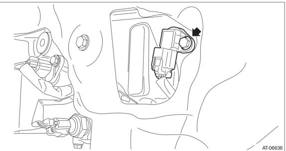
3) Remove the harness connector from primary speed sensor.
